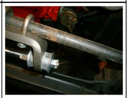
Turn the steering wheel completely to the left, then back about 1/4 turn. Orient the cylinder shaft bracket so the angled part (with the hole for the shaft) points forward, then slide the cylinder shaft bracket onto the cylinder shaft and attach the remaining shaft grommet, washer and nut. BE CAREFUL TO KEEP THE SHAFT EXTENDED. Tighten the shaft nut and insert cotter pin. Now tighten the cylinder shaft bracket nuts.
