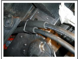
Insert both pump hoses through the bracket, adjusting the foam covers to protect the hoses as you pull the hoses through.
