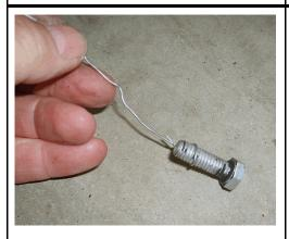
To install the pump hose clamp, wrap a thin wire around the attaching bolt.
