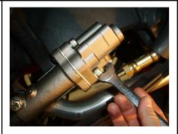
Attach both hoses to the valve. The SMALL hole in the valve is the PRESSURE port. The LARGE hole in the valve is the RETURN port.
