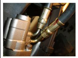
Pump hoses will be angled slightly to allow for full range of valve movement.
