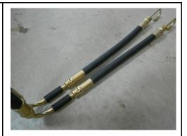
Find the long part of the L shape in the middle of the cylinder hoses and assemble hose grommets as shown.
