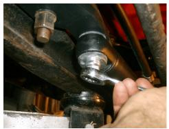
Install and tighten the large flat washer, lockwasher and nut on bracket stud.
