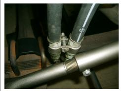
Orient hose clamp hardware as shown. This clamp will keep the cylinder hoses in an upright position.
