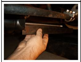
By hand, extend cylinder shaft completely out of cylinder.
