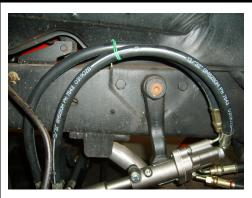
Attach the cylinder hoses to the valve. The hose on the cylinder closest to the FRONT attaches to the TOP valve connection, the REAR cyl hose attaches to the BOTTOM valve connection.
