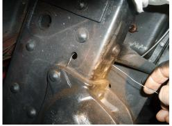
Find the hole in the frame side rail behind the rear leaf spring bracket. Insert the thin wire from the inside of this hole and pull bolt through.
