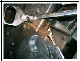
Attach the hose bracket onto the frame rail with provided nut and lockwasher. Orient the bracket as shown.
