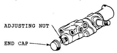
Pry off the end cap on the valve, under it is a 7/16" adjusting nut.
