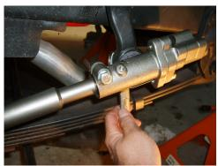
Install the valve assembly onto the pitman arm and the steering knuckle. Tighten nuts and insert cotter pins. Make sure valve stud at pitman arm is centered in the valve casting so it won't bind when operated.
