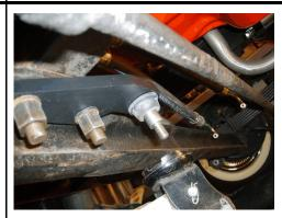
Install one of the cylinder grommets on the stud of the cylinder bracket.
