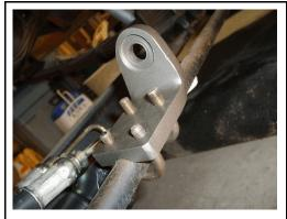
Place cylinder shaft bracket onto center link as shown and insert small U bolts.
