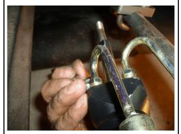
Attach the cylinder hoses to the cylinder. Use line wrench to snug hose nuts.
