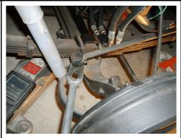
Remove the cotter pins and hardware at each end of the relay between the pitman arm and steering knuckle. Remove the old relay using a tie rod pickle fork.
