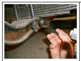
Remove both nuts on rear U-bolt of the driver side front axle assembly. Loosen the front U-bolt nuts.
