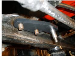
Underneath leaf spring, insert cylinder bracket onto rear U bolt, then reinstall all U bolt lockwashers and nuts.
