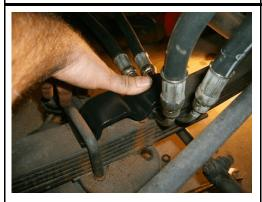
Install new spacer and hoses on top of leaf spring and place U bolts on top, orient slits in grommets on top. Use new U bolt at rear if needed.
