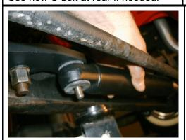
Install cylinder and the remaining cylinder grommet on bracket stud. Make sure the cylinder hose connections are ABOVE the shaft.
