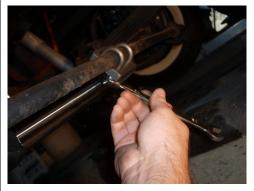
Orient U bolts on the back of the center link then loosely install all lockwashers and nuts onto U bolts, the bracket should be loose enough to slide along the center link. Don't install cylinder shaft onto bracket yet.
