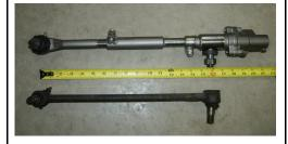
Assemble the valve onto the turnbuckle and assemble the relay onto the turn buckle. Measure the distance between the centers of the two studs, it should be about 15 ½ inches, verify by measuring your old manual steering relay. Orient the two studs to mimic the studs on your old manual relay. Tighten all hardware.
