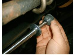
Install one shaft washer, the sleeve and one shaft grommet onto shaft. Be careful to keep cylinder shaft fully extended.
